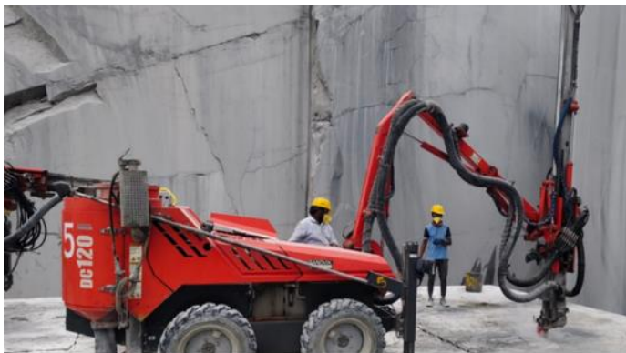
Drill machine equipped with dust sucking mechanism
