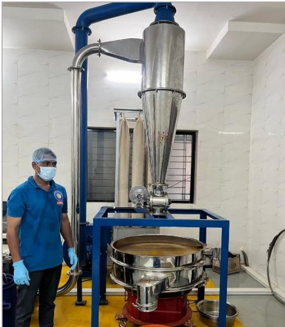
10-HP Masala Mill & Sifter Mesh Screen
